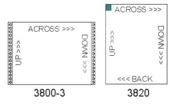
The 3800-3's media origin is at the left end of the long edge and the 3820's is at the left end of the short edge. Because of this different page definitions would be needed to print the same output on both printers. For example, in order to print landscape output an "across" page definition would be used on the 3800-3 and a "down" page definition for the 3820. This would require different page definitions to be specified for each printer.
