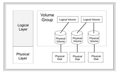
Each individual disk drive is logically represented by a physical volume (PV). Each physical volume consists of several partitions called physical partitions (PP). The physical partitions are grouped into something called a logical volume that contains logical partitions. The logical volume, in turn, belongs to a volume group. Logical volumes contain the file systems.
